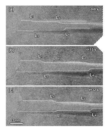
FIG. 2. A series of HRTEM images taken at different points of time (*t*), showing the twinning process at the Al crack tip. The TBs are outlined by dashed lines, and the progressing ledges on the TBs are indicated by  $L_1-L_4$ . (a) t = 0 s. (b) t = 15 s. (c) t = 32 s.
