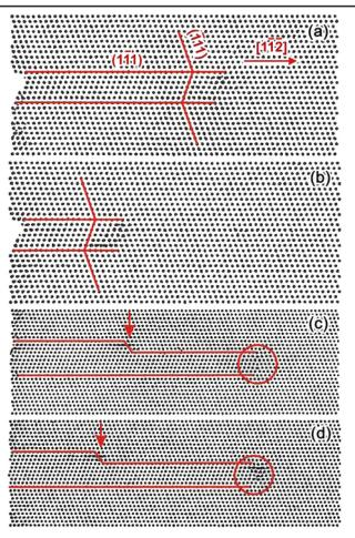
FIG. 4 (color online). (a) MD simulation model with [110] projection view; a six-layer twin ( $\sim$ 10 nm long) is embedded inside the matrix, with one end at the free surface. (b) Detwinning at 300 K. (c) A three-layer step created on top of a six-layer twin (left arrow) gradually moves towards the free surface. (d) As the position of the three-layer step changes, the six-layer twin boundary starts moving (right circle).
